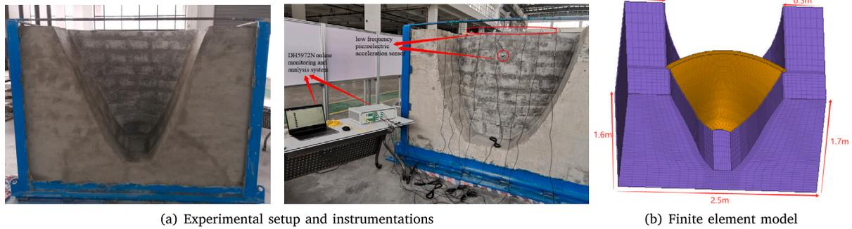
Fig. 10. Description of the small-scaled arch dam.
